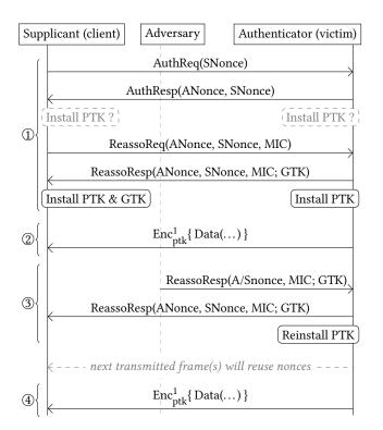
Figure 9: Key reinstallation attack against the Fast BSS Transition (FT) handshake. Note that a MitM position is not required, only the ability to eavesdrop and replay frames.
