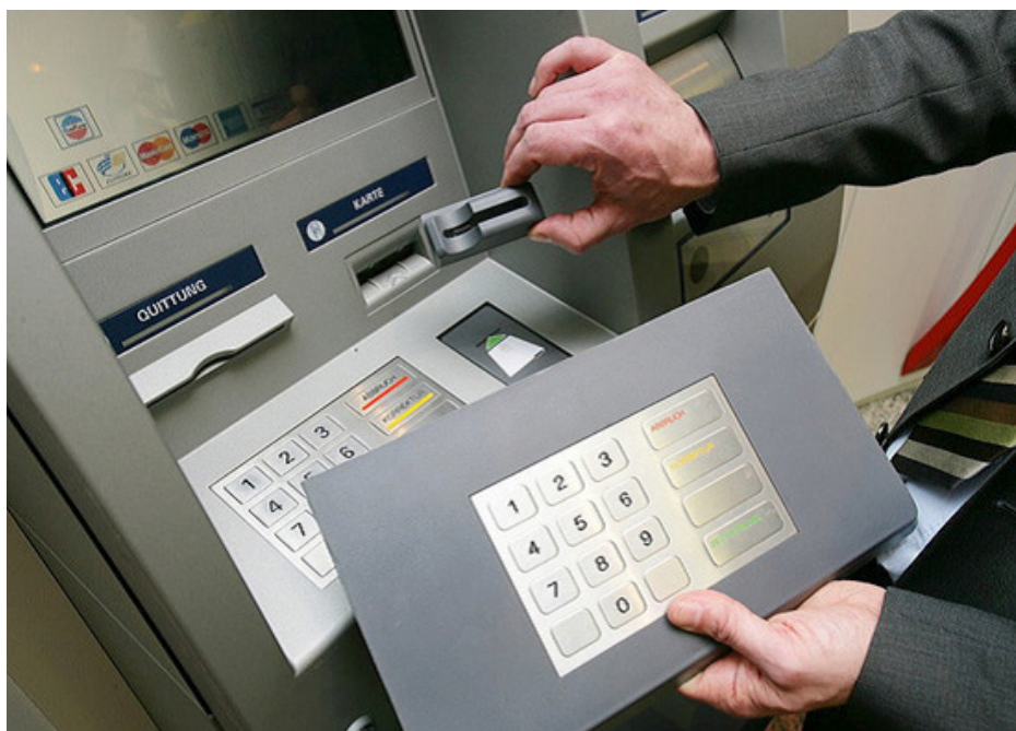
Figure 3. Old-school skimming attacks through physical means 8
