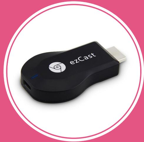
The device runs EZCast ROM (Linux OS) on a MIPS CPU and contains many apps created by the EZCast developers. Unfortunately, it also contains a number of easily exploited vulnerabilities.
