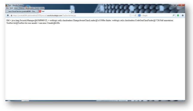
Fig. 3 Illustration of JSP file execution in the environment of Oracle Java Cloud Software ver. 13.2 indicating no enforcement of Java API whitelisting rules.
