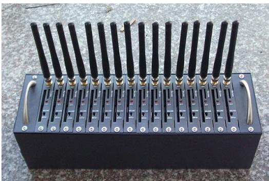
**Figure 3:** A GSM modem with 16 SIM card slots
