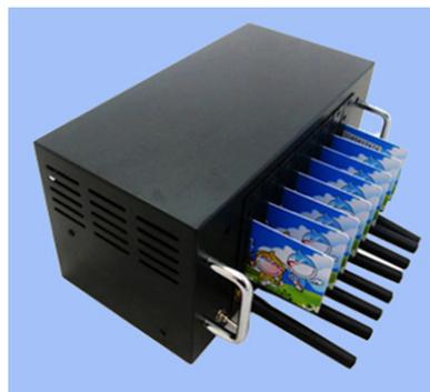
**Figure 4:** An 8-slot GSM modem with SIM cards
