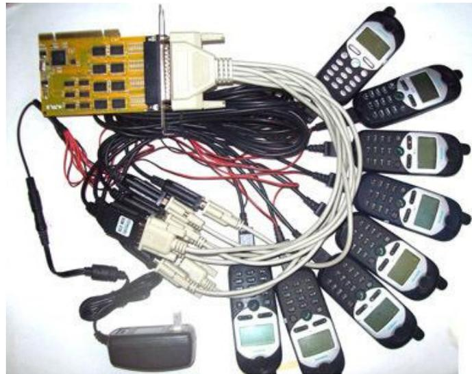
Figure 12: Eight GSM mobile phones can be connected to each serial card, all of which can be controlled by phone-number-scanning software
