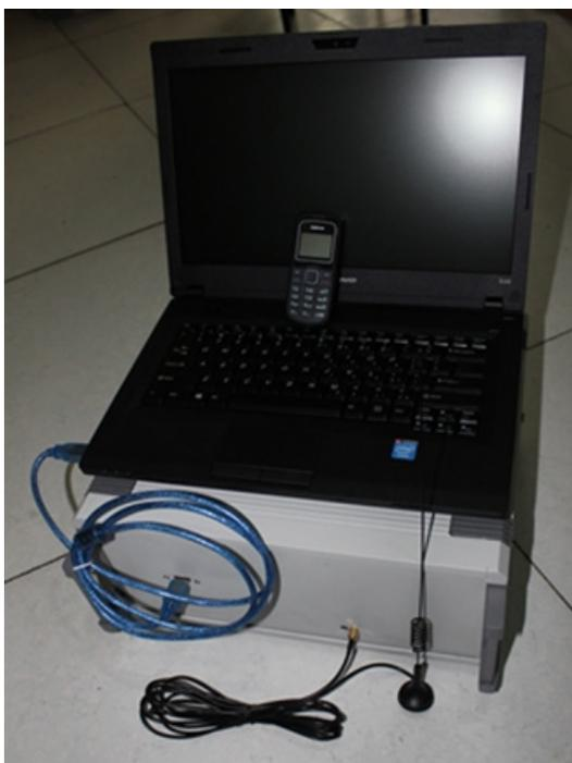
**Figure 5:** All-in-one SMS server package made up of a laptop, a GSM mobile phone, an SMS server box, an antenna, and a USB data cable sold underground for RMB 45,000 (~US\$7,400)
